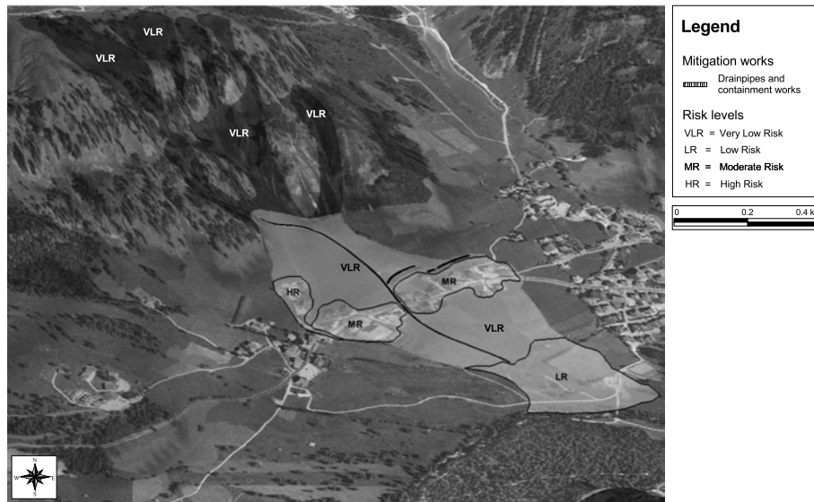
Fig. 8. 3-D representation of the spatial distribution of risk levels. Dark and light sectors symbolize the source and the depositional areas of the earth-debris flow, respectively (royalties on Digital Elevation Model and Digital Orthophoto: Autonomous Province of Bolzano-Autonomie Provinz Bozen-Sudtirol).
