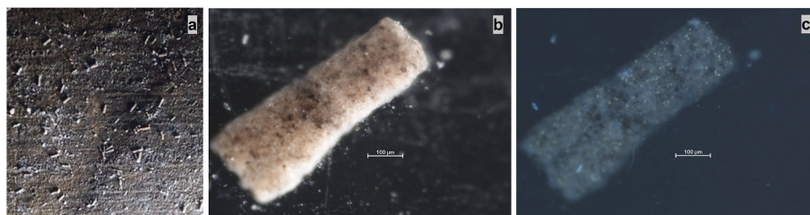
Fig. 5. The fecal pellets observed on site on the fresco surface under raking light (a) and in laboratory at a higher magnification under visible (b) and UV fluorescent light (c). Scale bar 100 µm.
