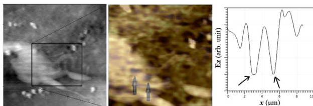
Fig. 1. (Left) 20 \mu\text{m} \times 20 \mu\text{m} topography of h9c2 mouse cells recorded with a homemade aperture SNOM. (Middle) Overlapping of the topography image with the corresponding optical map. The arrows denote the NS identified within the cell. (Right) Strong-absorption points marked by arrows in the overlapping image and denoting the dimensions of the NSs. (Adapted with permission from [10].)
