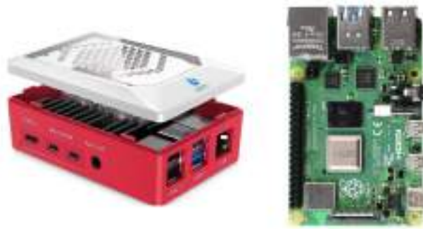
Figure 7. Elaboration unit (Raspberry Pi 4 Model B) for the acquisition and processing of sensory data and the fusion of high-level information classified by sensor nodes. Used case on the left and electronic board on the right.
