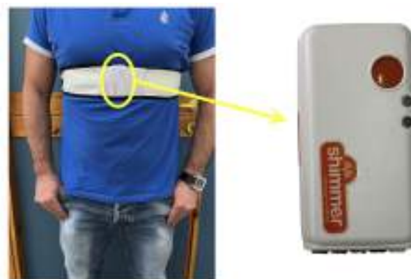
Figure 5. Wearable system integrating an elastic band (left) and Shimmer3 IMU inertial device (right) equipped with the following sensors: tri-axial accelerometer, magnetometer, pressure and temperature sensor and tri-axial gyroscope.
