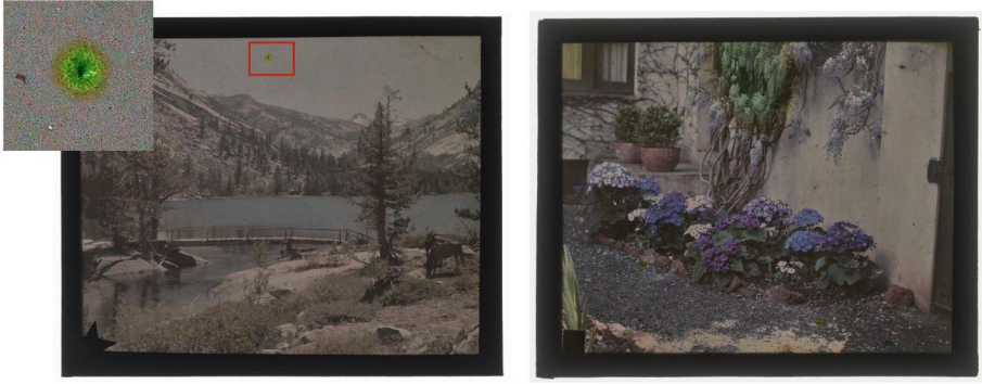
Fig. 44. Examples of real greening defects: small area or spotting defects (left) and large area defects (right). Image source [30].
