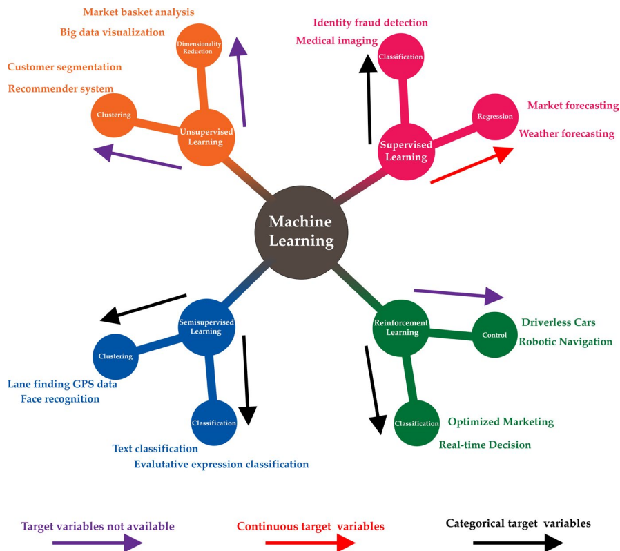
FIGURE 4 Machine learning. Different approaches to the learning process produce different machine-learning schemes. According to the number of features used to train the machine, one can obtain supervised learning (labelled data sets are used to train the machine), unsupervised learning (unlabelled data sets are used to train the machine), semi-supervised learning (a mix of labelled and unlabelled data sets are used to train the machine) and reinforcement learning (there are not data sets to train the machine). According to the quality of the target data (continuous or categorical), different tasks can be performed by the learning processes
