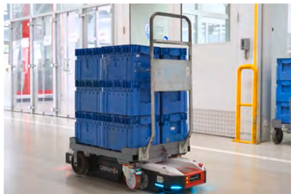
Fig. 1. Prototype of the omnidirectional AGV carrying a cart in the manufacturing industry.
