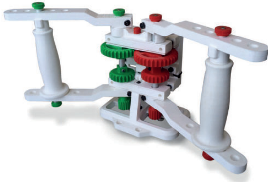
Figure 1. DUALarm—a low-cost, open-source and 3D-printable device for upper limb neurorehabilitation.
