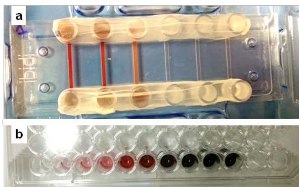
Figure 5: a) photograph of a plastic device with three of its six micro-channels filled with blood and two different dilutions of gold nanorods in blood; b) photograph of a 96-well plate filled with different dilutions of gold nanorods in PBS.
