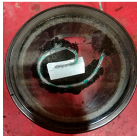
Figure 2. Piston window instrumented with a K-type thermocouple [17]. Reprinted with permission from ref. [17] Copyright 2019 SAE International.
