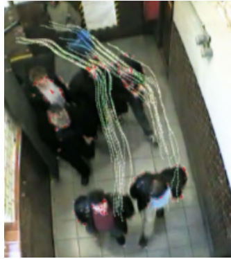
Figure 2.2: Example of clustering by motion similarities [34]. The assumption is that a pair of points that appears to move together is likely to be part of the same individual.
