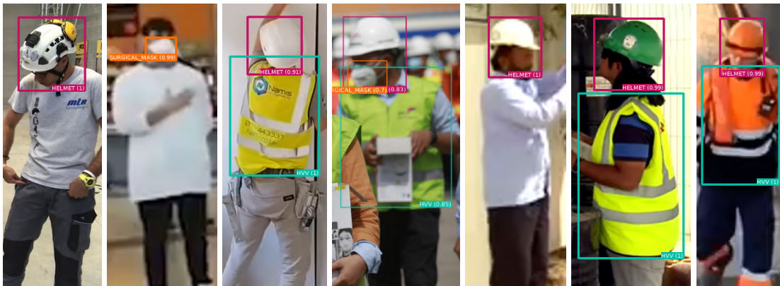
Figure 7.7: Examples of predictions of the PPE Detection module on our CrowdVisorPPE test set. PPE classes are color coded ( helmet , high-visibility vest , face mask ), and the detection score is reported in parenthesis.
