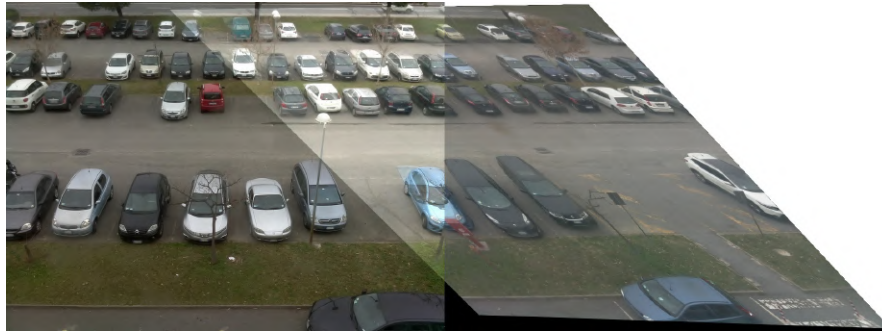
Figure 3.7: Example of concatenation of two images using a homographic transformation. It is also visible the overlapping area between them.
