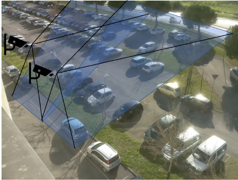
Figure 3.5: An example of two cameras monitoring the same parking area with partially overlapping fields of view. This redundancy provides robustness and fault-tolerance, but it also raises the problem of aggregating knowledge extracted from the individual cameras.
