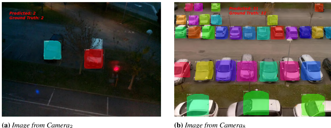
Figure 3.8: Examples of vehicle localization and counting in the Single-Camera Scenario. Images are taken from the CNRPark-EXT dataset. We report the masks localizing detected cars and the estimate of their number.
