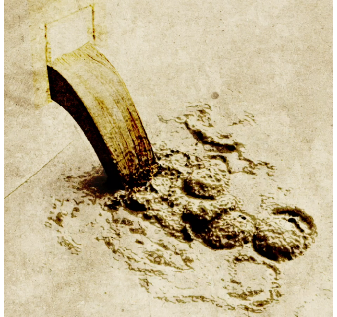
Fig. 9. SPH simulation using an air-water model. Non-photorealistic rendering, 3D view from the top at time instant 5.8 s.
