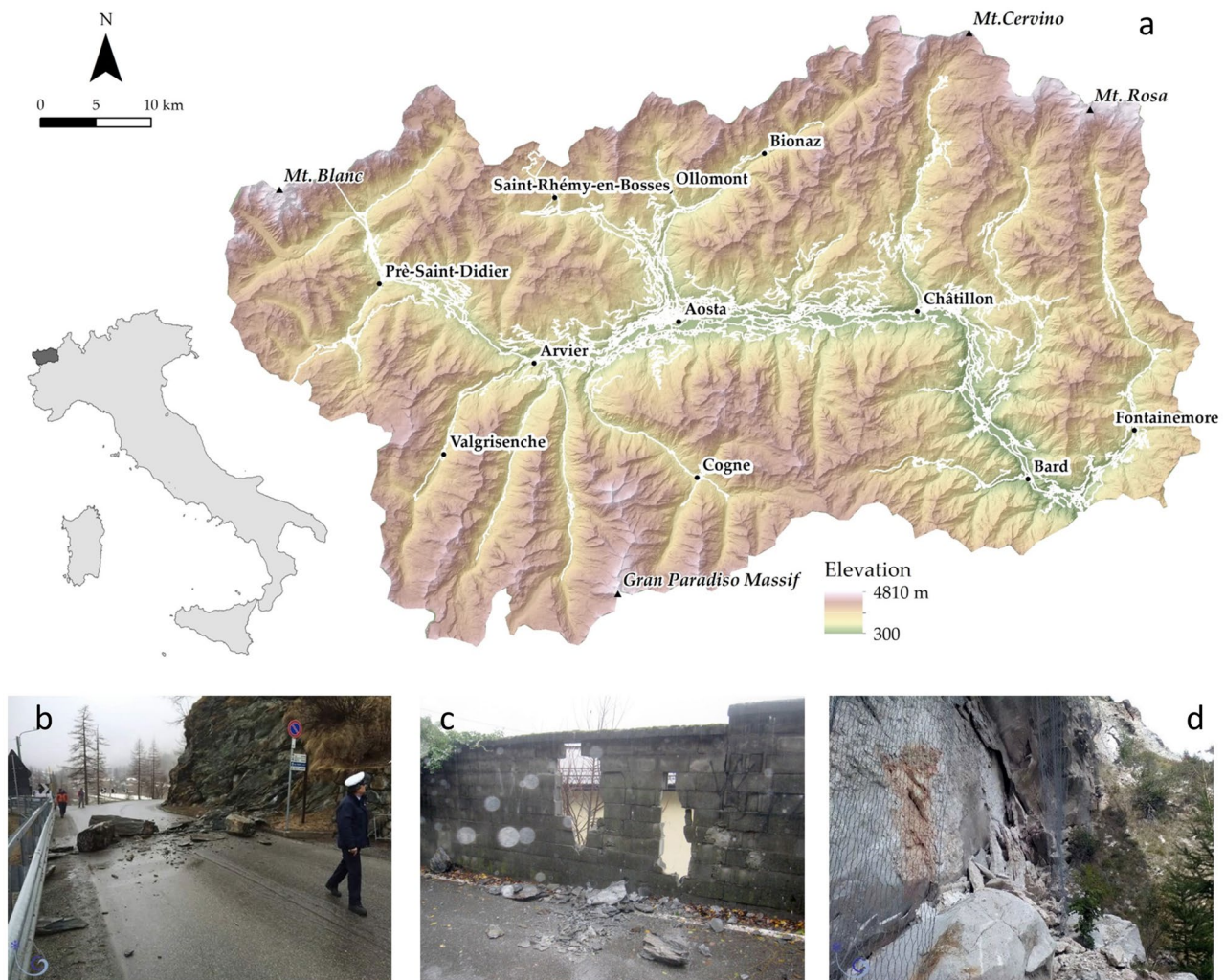
Fig. 1 (a) Relief terrain map of the Aosta Valley mountainous territory (north-western Italy), associated to the elevation map, showing the extended road network (white polylines), branched along the main valley of this alpine region highly affected by rockfalls that cause relevant damage to (b) road pavement and vehicles, (c) urban settlements, and (d) existing structural protective measures
