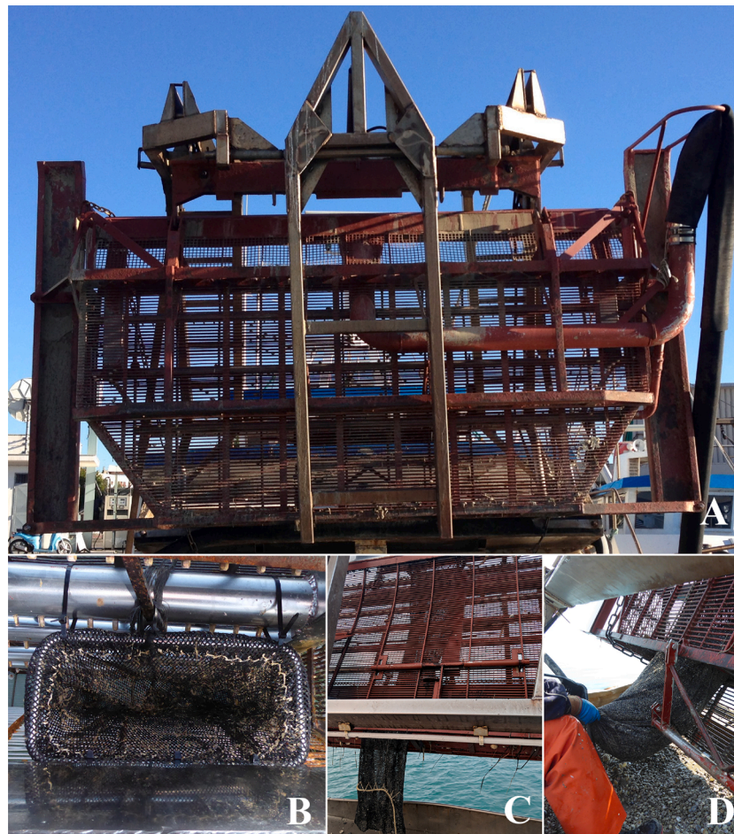
Fig. 2. Illustration of hydraulic dredge targeting Chamelea gallina and details of the net sampler used as a control to assess the size selectivity of the dredge: (A) metal cage located at the bow; (B) particular of the steel frame (40 × 18 cm) fixed inside the dredge mouth; (C) lateral view of the net sampler inside the cage; (D) emptying of the net sampler.
