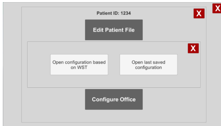
Figure 7: The new interface. It is now possible to close each window separately and easily return to the previous step. The labels on the buttons make the interaction more intuitive.
