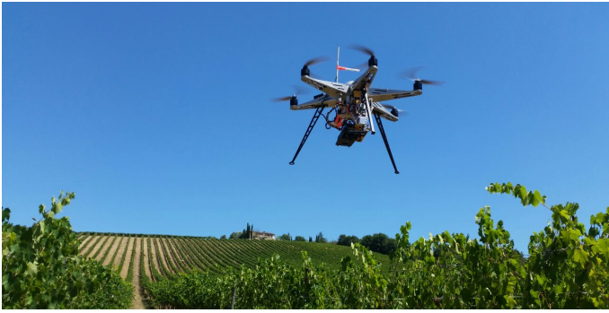
Fig. 1: EFESTO is an UAV developed by CNR, mounting a thermal imaging camera, a multi-spectral snap, and two hyper-spectral fiber optic sensors for smart farming applications.
