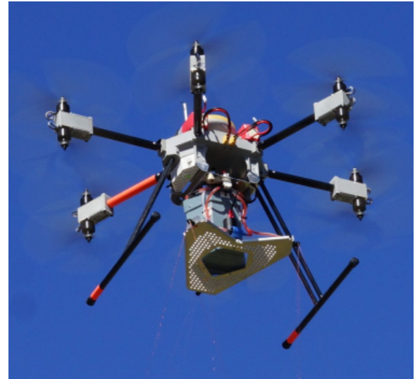
Fig. 2: Treatment of the processionary moth by a second UAV made by CNR. Three precision sprayers are mounted at the edges of the UAV payload.
