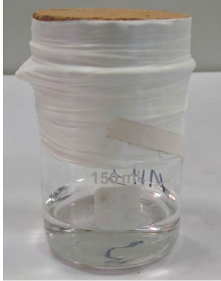
Fig. 6 Earthen samples were fixed on the top of cylindrical containers that are partially filled with water, sealed with a polytetrafluoroethylene tape, to evaluate the water vapour transmission
