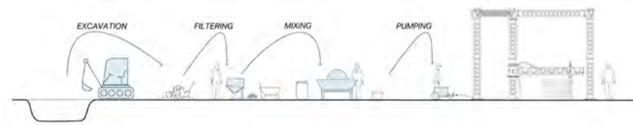
Fig. 5 Diagram of material feeding system by WASP, 2018
