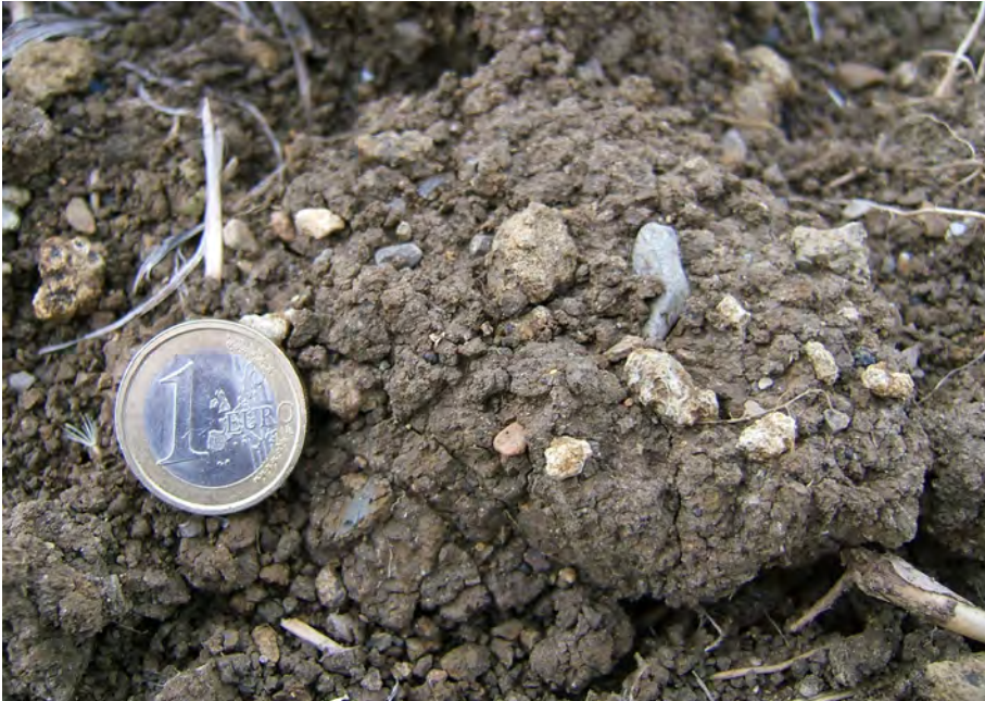
Fig. 1 Particular of an earth, it is possible to recognize the different grain fraction and the organic component
