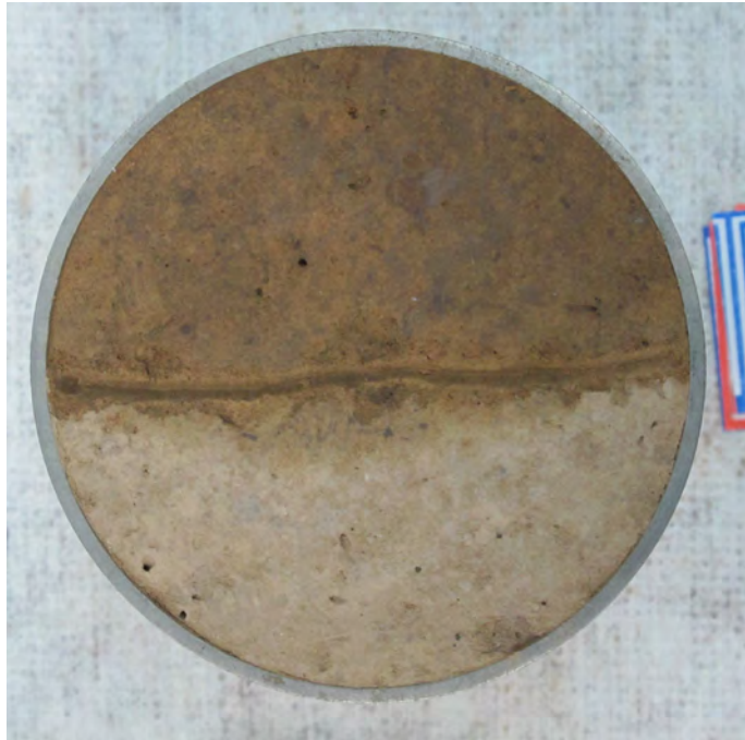
Fig. 5 Earthen samples are divided with a scored line and the consolidant is applied to one half. After curing of the consolidant, the colour difference between the two parts is evaluated to decide the gray scale rating
