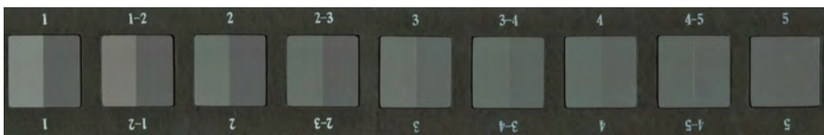
Fig. 4 Grayscale for assessing change in colour (from China standards GB 250-2008)
