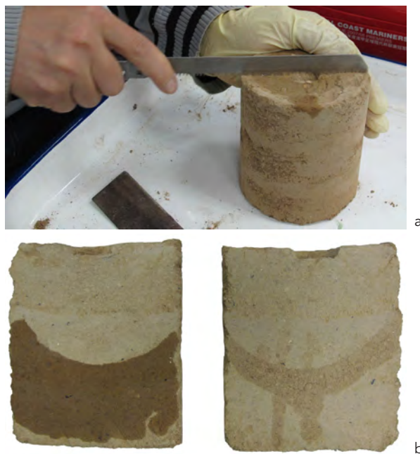
Fig. 3 Earthen samples ( \varnothing 100 mm \times 120 mm) made for the measurements of the treatment depth: a) earthen samples cut into two halves; b) some water is put in one half the upper dry part means that is consolidated, the lower wet part is unconsolidated (left). The right image is after water evaporation.
