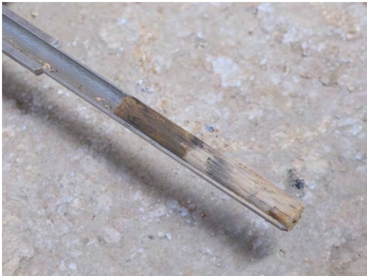
Fig. 8 Measurement of the depth reached by the consolidating treatment in the field immediately after application: trace of consolidating liquid in the sampling pipe
