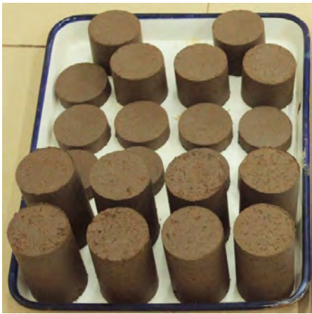
Fig. 5 Remoulded sample blocks at different heights
