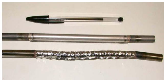
Fig. 6. Pd–Ag thin wall permeator tubes: as produced (above) and after testing (below).
