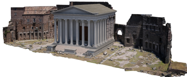
Fig. 10. 3D reconstruction of the Temple of Mars Ultor juxtaposed with the 3D model of the site digitised with IBM techniques
