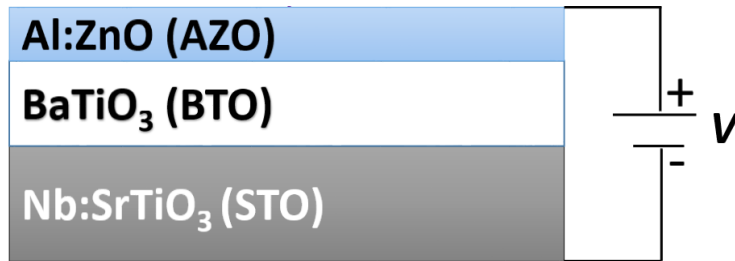
FIG. 3. Three-layer system used for spectroscopic ellipsometry modeling. The variations in the carrier density of AZO ( N_e ) upon dc gating (0.1-0.5V) were calculated.
