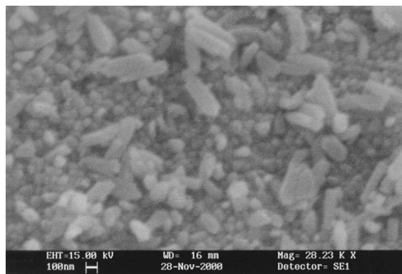
Fig. 2. Top view of the 50 nm \alpha\text{-Al}_2\text{O}_3 support (SCT) after the preparation of the MFI 50(1) membrane.
