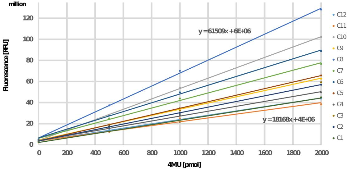
Figure 2: The x-axis shows the total amount of fluorescent 4MU molecules in the calibration wells and the y-axis shows the corresponding fluorescence. The colored lines represent the calibration curves for each sample. The angular coefficient, resulting from linear regression, is the  $\alpha$  coefficient used to calculate enzyme activities with the first method. The slopes of the different calibration curves differ significantly from sample to sample.
