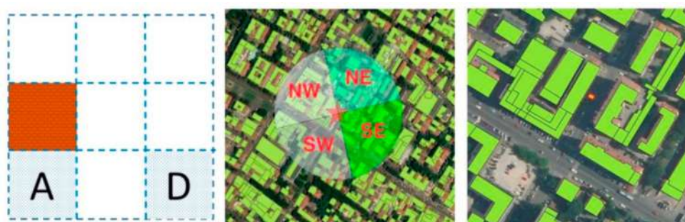
Figure A1. Left: positions of the A and D points with respect to the CT indicated here with the brown square. Centre: sectors considered according to the viale Verdi orientation. Right: position of the CT, in red, and the buildings and streets nearby.
