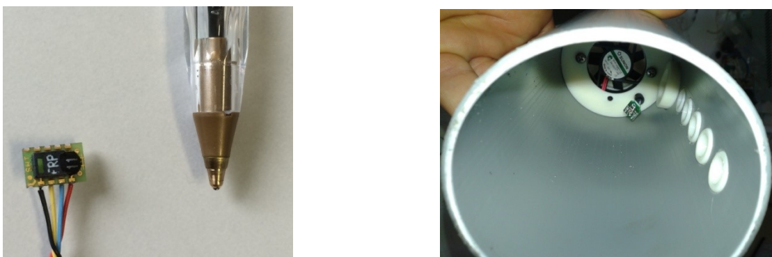
Fig.17. Sensirion SHT11 temperature sensor, left, and its location inside the store chamber, right.
