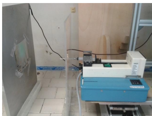
Fig. 38: Electrospinning set up comprising a syringe fitted with a blunt tip needle and a metallic screen as fibers collector
