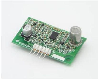
Fig. 11. Electronic module for this gas sensor: AM-4-4161 from Figaro Engineering.
