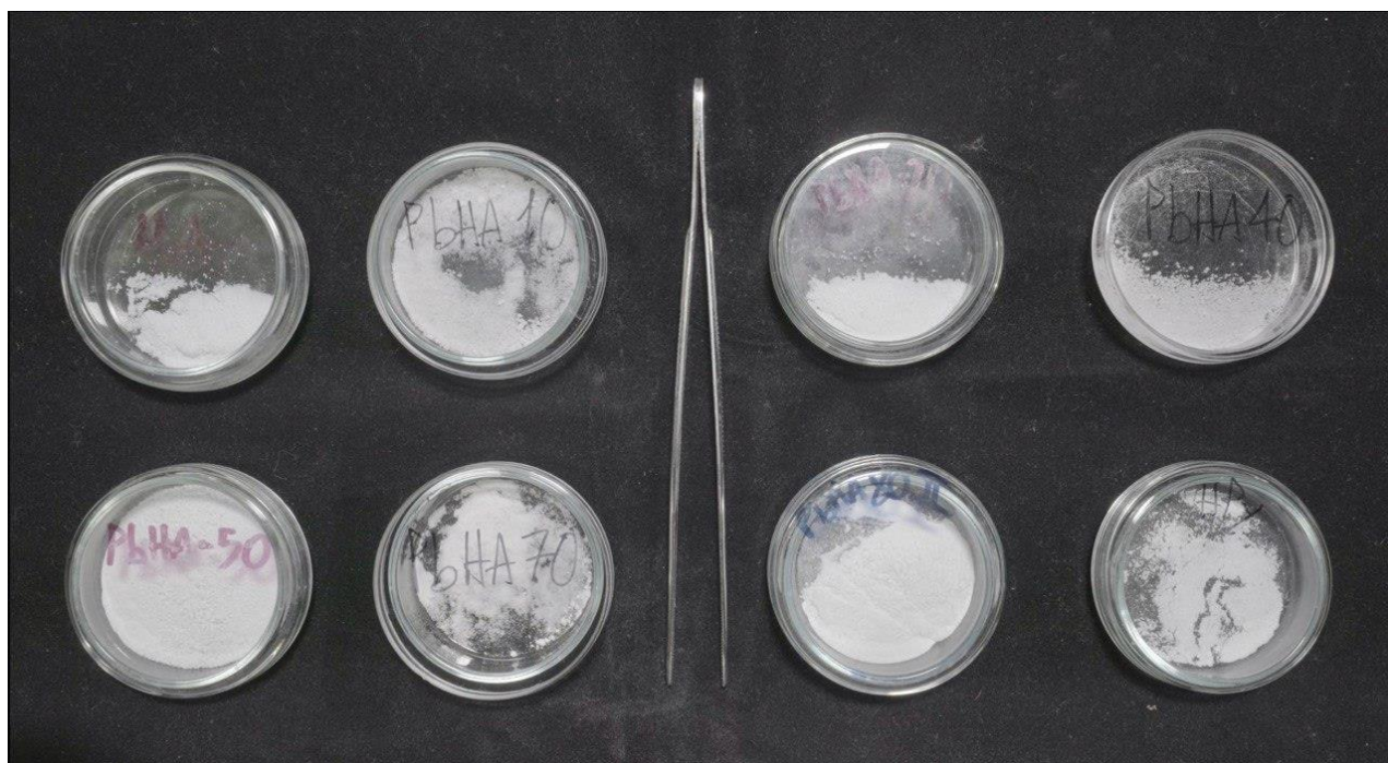
Figure 3.1 Photograph of the complete set of the synthesised \text{PbHA}_x compounds. From top left: HA, \text{PbHA}_{10} , \text{PbHA}_{20} , \text{PbHA}_{40} , \text{PbHA}_{50} , \text{PbHA}_{70} , \text{PbHA}_{80} and HPy.
