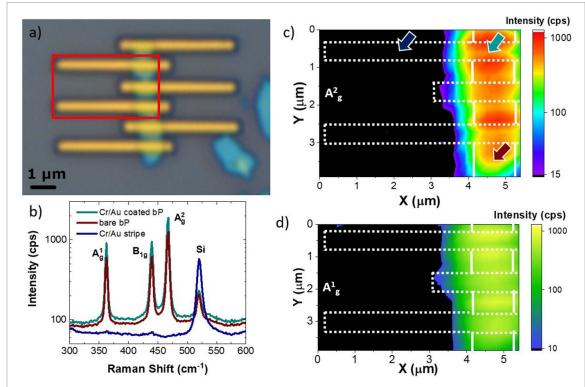
**Figure 3.** (a) Optical image of a bP flake with Cr/Au stripes. The red square indicates the area where the Raman maps were acquired. (b) Raman spectra acquired on the bare bP (red line), on the Cr/Au coated bP (cyan line), and on the Cr/Au stripe at 1  $\mu$ m away from the bP flake (blue line). The area of collection are highlighted by colored arrows in (c). The same color code as for the spectra is employed. (c) Intensity map of the  $A_g^2$  mode. (d) Intensity map of the  $A_g^1$  mode.
