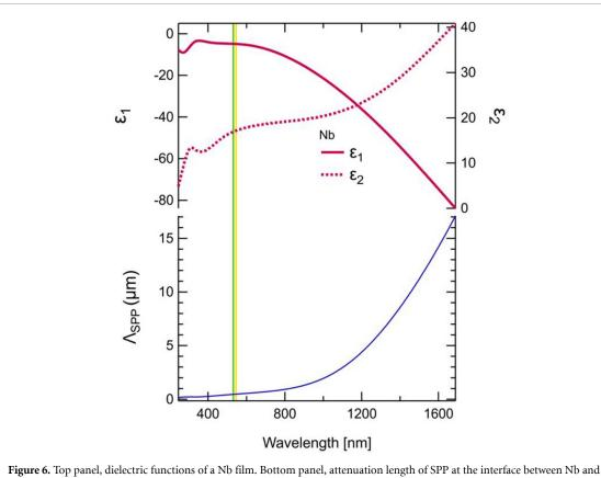
PMMA. The vertical green line is at  $\lambda = 532$  nm (excitation), while the yellow line is at  $\lambda = 546$  nm (Raman).
