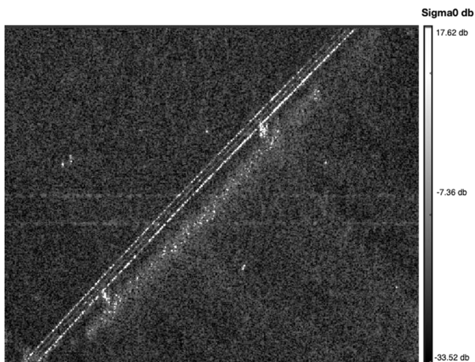
Figure 7. Backscatter intensity at Baishazhou Bridge, from COSMO-SkyMed StripMap HIMAGE SAR scene acquired on 13 July 2016. COSMO-SkyMed® Products ©ASI—Italian Space Agency—2016. All rights reserved.
