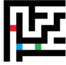
Fig. 4. The state [(10; 10; 0)\_\#FFFFFF, (5; 7; 0)\_\#FFFFFF, \text{Driver}, \text{Close}] of the composition of two agents, a driver, and a door. The door is in position (2; 7) and is closed. The first agent is depicted red, the second is green, and the door is blue. The attributes of the position of the two agents are both \#FFFFFF , which is the hexadecimal value for the colour white, i.e., both agents are placed on a white cell of the map.
