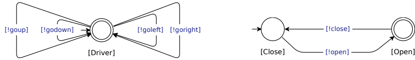
Fig. 3. The driver automaton on the left, the door automaton on the right
