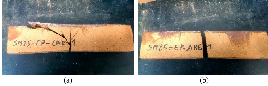
1 Figure 9. Typical failure of FRP reinforced brick specimens: debonding/shear (a) and fibre tensile 2 rupture (b)
