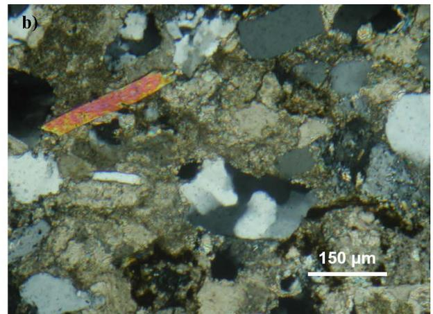
Figure 10. a) Ternary diagram (quartz, feldspars, rock fragments- modified after Folk, 1974) representing the petrographic classification fields of Pietraforte (violet) compared to Pietra Serena (green); b) thin section photomicrograph of Pietraforte sandstone: here is visible the clastic fraction made of quartz, micas, dolomite rock fragments and the matrix made of the micritic carbonates mixed with clay minerals (transmitted light, xpl).
