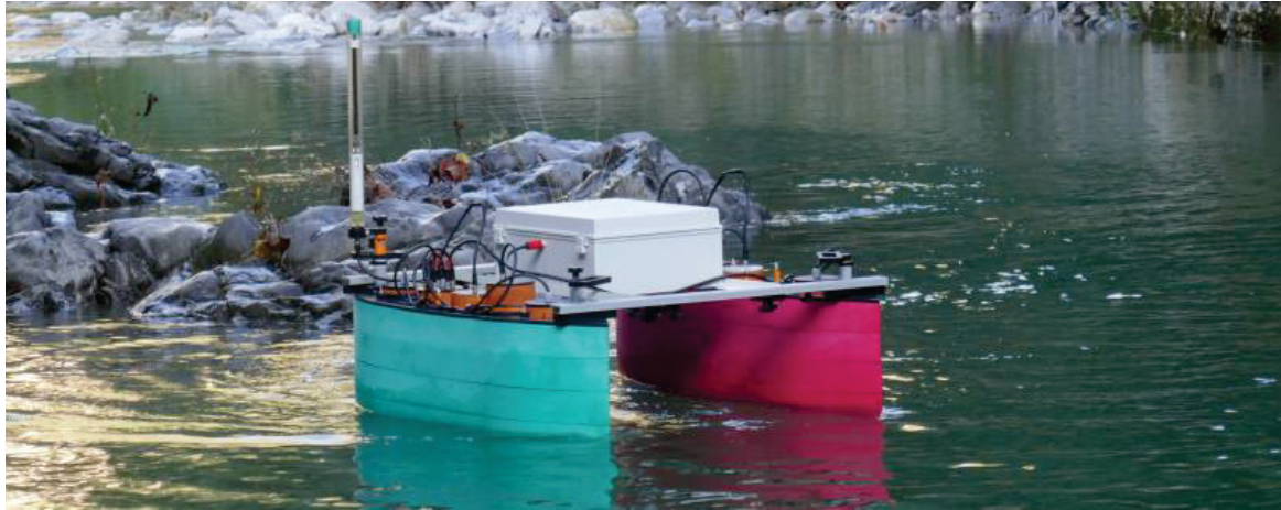
Fig. 1 - SWAMP vehicle during a survey with a payload box on the deck
