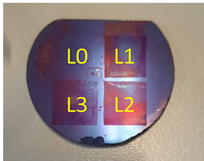
Fig. 1. Laser-processed \text{LaB}_6 ceramic disk. L0: pristine untreated surface. L1-L3: treated surfaces.
