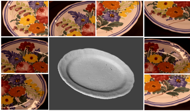
Fig. 4. The dataset used for the test (3D model and all eight images), representing a ceramic dish.
