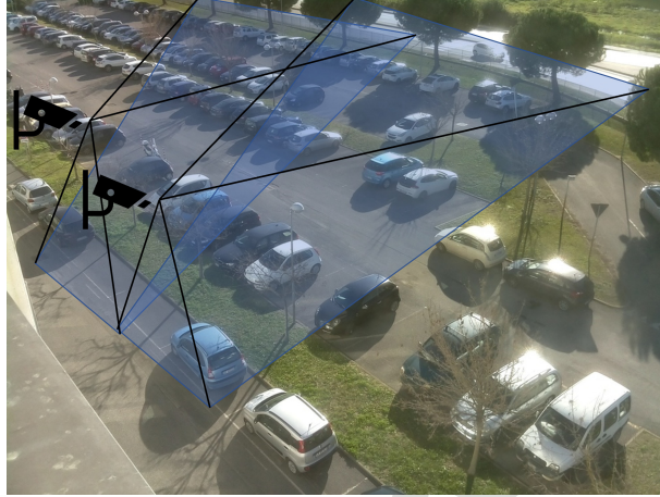
Figure 1: An example of two cameras monitoring the same parking area with partially overlapping fields of view. This redundancy provides robustness and fault-tolerance but also raises the problem of aggregating knowledge extracted from the individual cameras.
