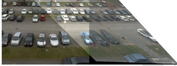
Figure 3: Example of concatenation of two images using a homographic transformation, where it is also visible the overlapping area between them.
