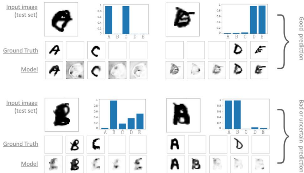
Fig. 3. Examples of prediction of our deep learning model: in the top panels the segmentation of complex combinations of A + C and D + E ; in the bottom panels the segmentation of complex combinations of B + C and A + D .
