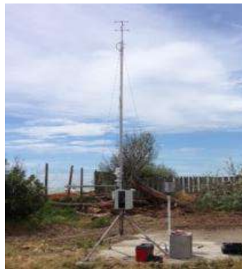
Figure 3. The micro-meteorological station with an ultrasonic anemometer–thermometer, thermo-hygrometer, net-radiometer, barometer, and pluviometer. The instrumentation is specified in Table 1.
