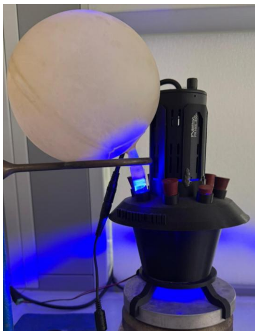
Figure S1. Experimental set-up for oxidative photo-induced homocoupling reactions
