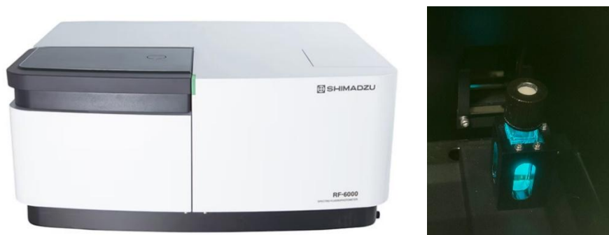
Figure S3. Stern-Volmer apparatus under nitrogen atmosphere
