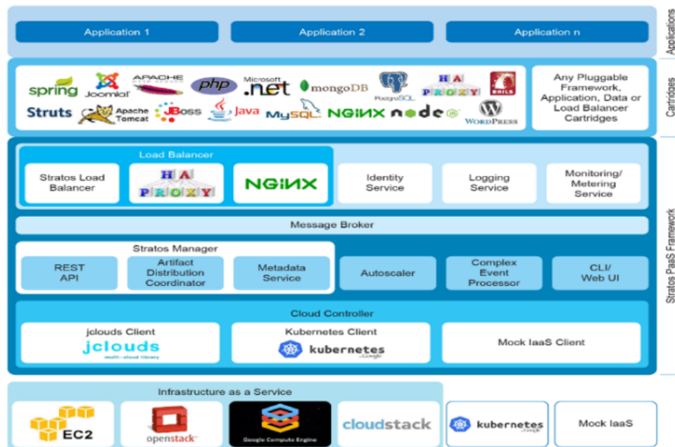
Figure 9. Architecture of Stratos [Source: apache Stratos, 2015]
