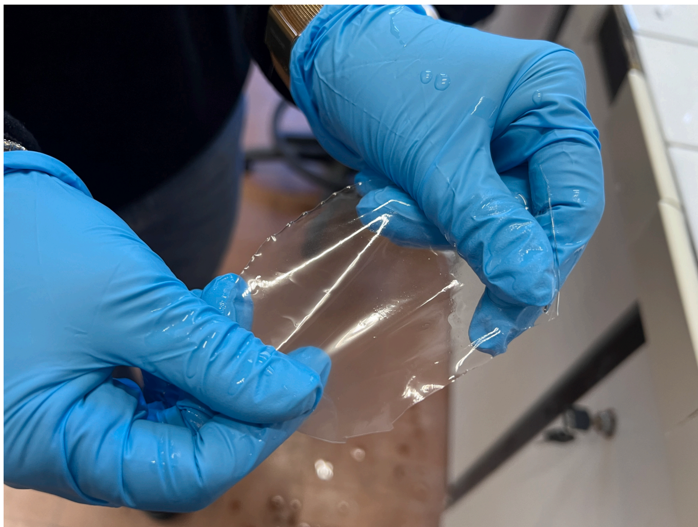
Fig. 4. Lemon CytroCell@PIL anion exchange membrane (photo courtesy of M. Pagliaro).
