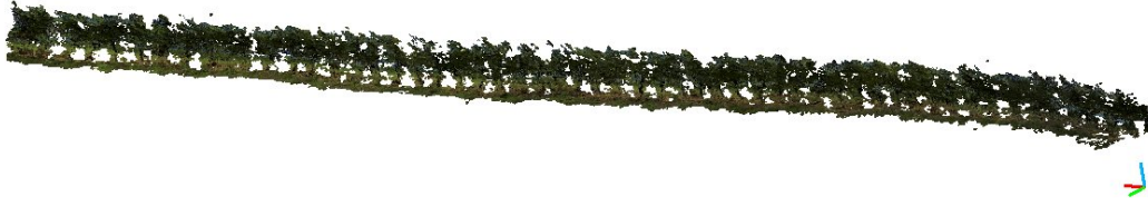
Figure 9: 3D reconstruction of the grapevine row under inspection. It includes 55 plants spanning along a total length of approximately 50 m. Plants are located at approximately 0.90 m apart with respect to each other.
