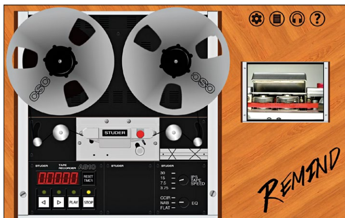
Fig. 5 – The main activity of REMIND app. A video of the original tape is shown outside the body of the tape recorder to improve its readability.
