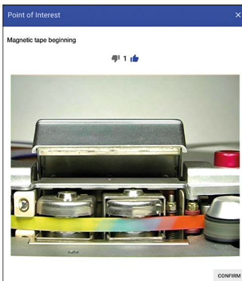
Fig. 4 – A POI pop-up with a frame of a splice correctly detected. The technician in the digitizing lab can confirm or reject the correctness of the result.
