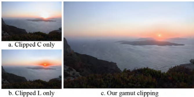
Fig. 8: Three different clipping solutions were used to process the same image. Since most of the out-of-gamut pixels reside in the top right corner of the cusp, clipping along only the chroma direction (a) severely desaturates these pixels. In contrast, clipping only along the lightness direction (b) leads to an unnatural, oversaturated appearance. The result of our interpolated solution is shown in (c), where the image has maintained a natural appearance while all pixels fit within the gamut boundaries.
