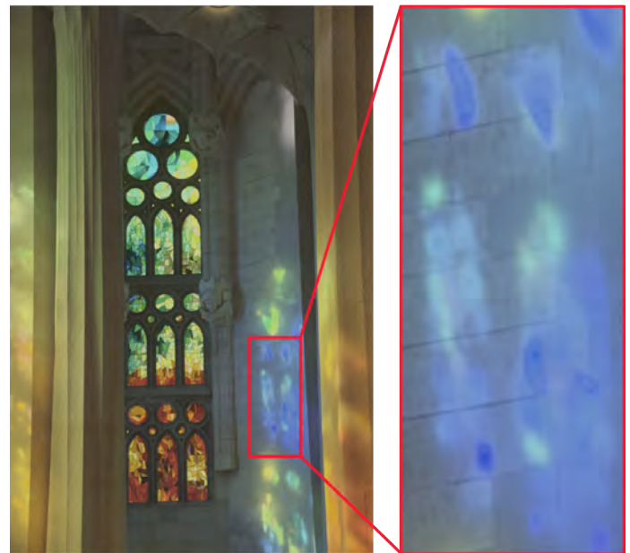
Fig. 13: An example showing that the SCACLIP gamut mapping method [9], integrated with an existing TMO [8] may introduce artifacts.
