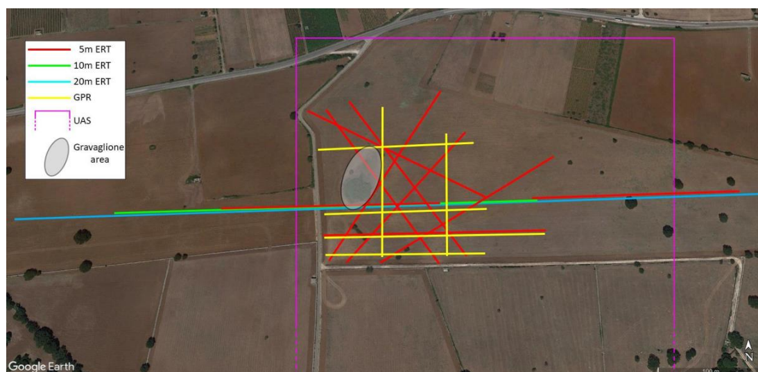
Figure 5. Geophysical survey in the area surrounding the Gravaglione swallow hole.
