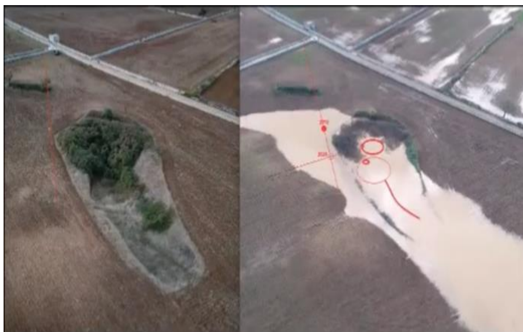
Figure 4. The Gravaglione swallow hole after a rainstorm in December 2020. Red circles highlight the main adsorption areas and the water entrances to the underground (photo courtesy by Rodrigo Torres).
