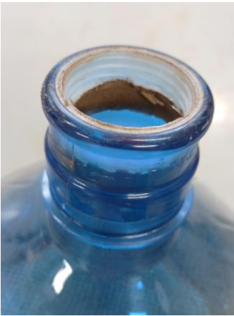
Fig. 5. The perforated cap is glued to the inside of the funnel base.
