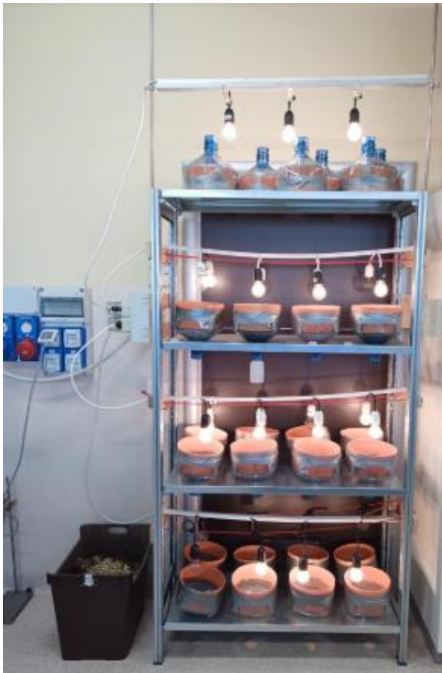
Fig. 8. To allow the simultaneous extraction of multiple samples, a shelf with twenty-seven positions distributed over four tiers has been created. The structure was made using a metal shelf measuring 40x100x200, whose tiers were drilled with a column drill and a hole saw (hole diameter 8 cm) to support the traps. Each level accommodates 8 traps, except for the last one, which holds 3.
