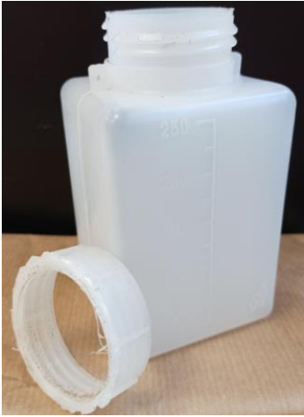
Fig. 4. The 250 ml container, filled with approximately 40 ml of an alcohol and glycerin-based solution, is screwed beneath the funnel using the threading of its perforated cap, which is glued inside the funnel (see Fig. 4).
