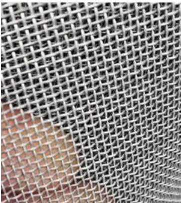
Fig. 2. The metal mesh used to create the sieve was hand-cut into a circular shape with a diameter of 220 mm using tin snips. It was then shaped and secured to the inner base of the orange PVC pipe with screws and glue. The mesh has 2x2 mm square openings, which effectively hold the soil clump above while allowing microorganisms to pass through, thus acting as an efficient filter. This type of mesh is sold by the meter at stores specializing in steel materials.
