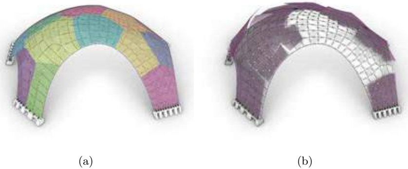
Fig. 10. Minimum distortion patches of wire mesh to lay on the top face of the shell: (a) developable patches; (b) flat sheets of material.
