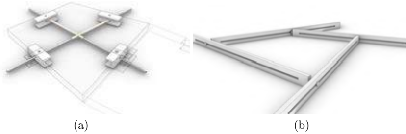
Fig. 6. (a) Detailed design of the prismatic tile with embedded cables' ducts and steel C-profile segments at the contact interfaces. (b) Adaptable molding system.
