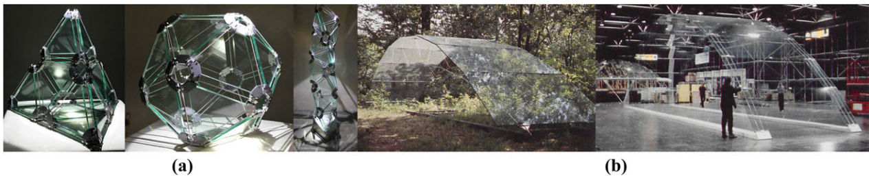
Figure 2: (a) Mock-ups of structures with structural glass [FL18] and (b) arches with structural glass [Sob07].
