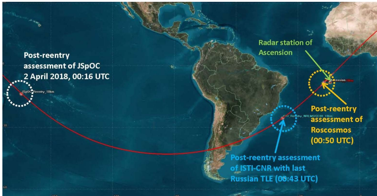
Fig. 22. Post-re-entry assessments of Roscosmos and ISTI/CNR, at the “conventional” altitude of 10 km (IADC), based on the last Russian orbit, compared with that of JSpOC, based on the last US TLE.
