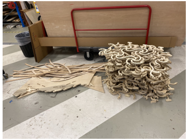
Figure 18: Fabrication of the demonstrator: CNC cutting and components after sanding
