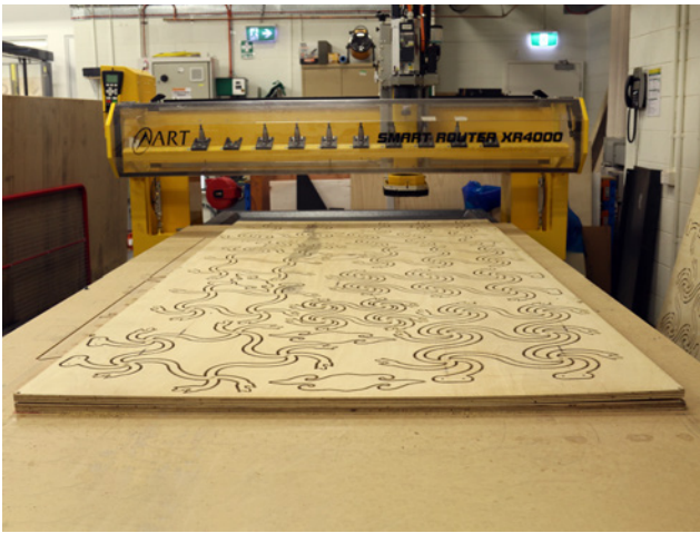
Figure 18: Fabrication of the demonstrator: CNC cutting and components after sanding
