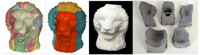
Figure 10: An example demonstrating the multi-piece molds generation algorithm from Herholz et al. [HMA15]. From left to right: the output of the method when no undercut constraint violations are allowed, the regularized output with surface deformation, the resin cast, and the mold pieces.
