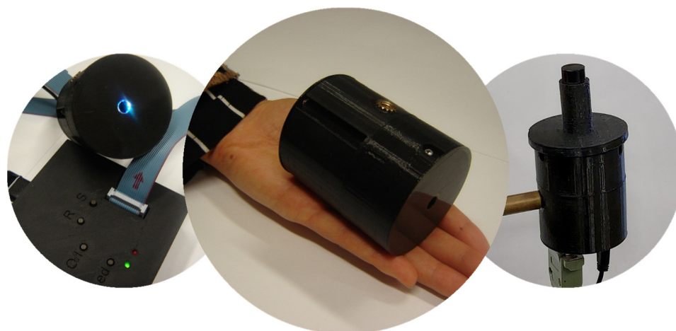
Figure 7. The fluorometer (center), with the supply unit (left) and with the vial holder (right).
